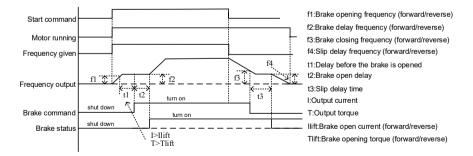
Brake is the most crucial and most important institutions of crane system. Reliability of brake relates to safety of whole machine. Except the brake control time sequence to ensure reliable
