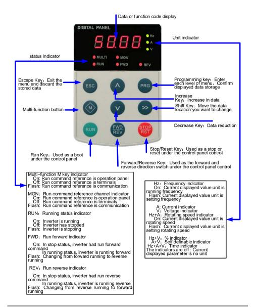
With a 9-button operation panel and a shuttle-type operation panel, the two operation panels are fully compatible and can be selected at will.
