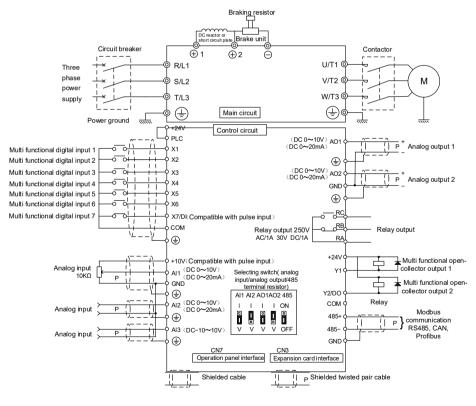
Figure 2-2 Terminal wiring diagram
